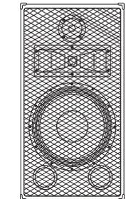
The speaker-system may only be installed on a stand or speaker stand if the original speaker-system is equipped with an appropriate flange.
