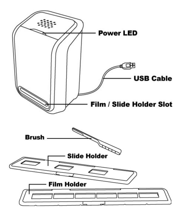
**Note**: We strongly suggest using the supplied Clean Brush to insert into the reflecta x8-Scan slot and clean the glass surface periodically to produce a clear image. Please make sure your film negatives/ mounted slides and cover trays are clean before inserting into the copier as well. Dust or dirt from the negatives and cover trays will affect the quality of your scanned images.
