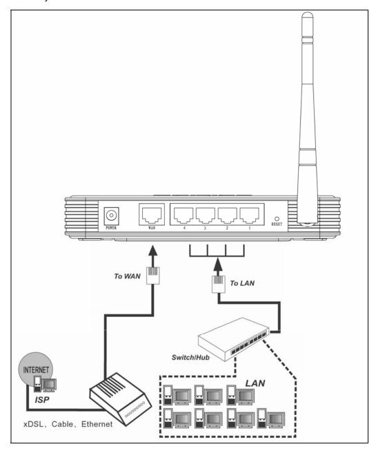
Figure 2-1 Hardware Installation of the TL-WR740N Wireless Lite N Router
