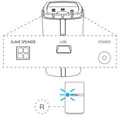
MM-1 connection sockets are found on the back and the underside of the powered speaker. Those on the underside are the **power input** socket, the **USB** socket and the **slave speaker** socket. Those on the side are the **line input** socket and the **headphone** output socket. The connection sockets are illustrated above.
