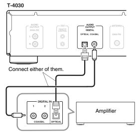
Use the digital audio cable to connect the T-4030's DIGITAL COAXIAL/OPTICAL jacks to the DIGITAL IN jacks on your amplifier, as shown.
