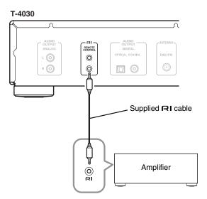
To use the  $\square$  system functions, use the supplied  $\square$  cable to make an  $\square$  connection (see the next column).
