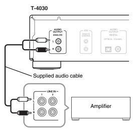
Use the supplied audio cable to connect the T-4030's AUDIO OUTPUT L/R jacks to the LINE IN jacks on your amplifier, as shown.
