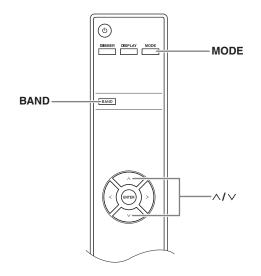
Use the tuner's [BAND] button, or the remote controller's [BAND] button to select FM.
