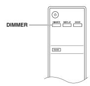
Press the remote controller's [DIMMER] button repeatedly to select: dim, dimmer, or normal brightness.
