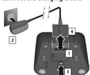
▶ To remove, press the release button 3 and disconnect the plug 4.
