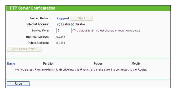
Figure 4-35 FTP Server Configuration
