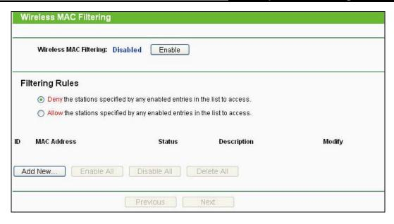
Figure 4-22 Wireless MAC Filtering
