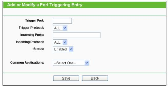
Figure 4-52 Add or Modify a Triggering Entry
