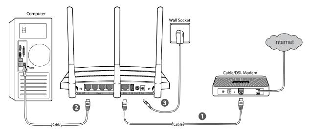
Figure 2-1 Hardware Installation of the 300Mbps Wireless N Gigabit Router
