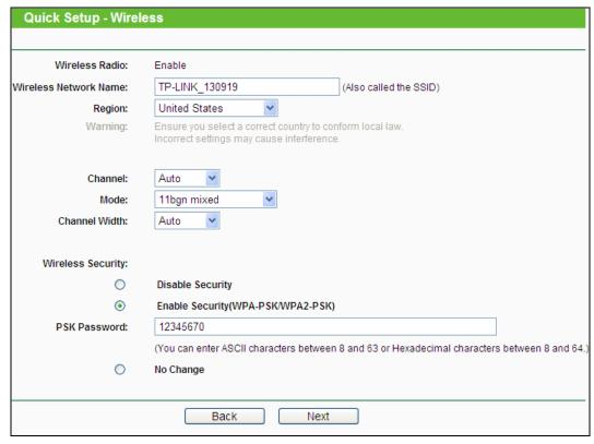
Figure 3-12 Quick Setup – Wireless
