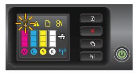
The printhead is incompatible or damaged.
