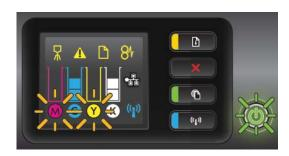
One or more of the ink cartridges are faulty, need attention, incorrect, missing, damaged, or incompatible.
