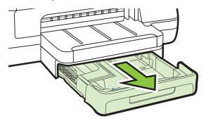
2. Insert the envelopes print-side down and load according to the graphic. Make sure the stack of envelopes does not exceed the line marking in the tray.
