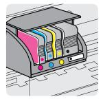
Make sure that you insert the ink cartridge into the slot that has the same colored letter as the color you are installing.
