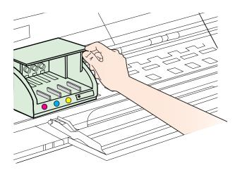
**4.** Remove the printhead by lifting it up and then pulling it out of the printer.
