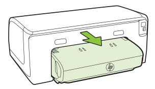
Reinsert the duplexer into the printer.
