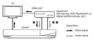
\* This connection is unnecessary for connection (HDMI connection).
