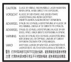
Pick-up unit of this appliance is classified as a CLASS 3R LASER product. Visible and invisible laser radiation is emitted when the laser protective housing is opened, so be sure to avoid direct eye exposure.
