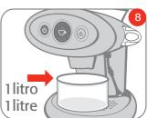
Press the coffee switch  $\bigcirc$  to start the decalcification cycle the coffee switch  $\bigcirc$  turns off  ${\bf 5}$
