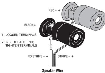
Figure 4. This figure shows how to connect bare wires to the terminals.
