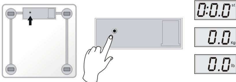
You can change the units among kg, lb, st by pressing the button on the back of the scale when it is power on.
