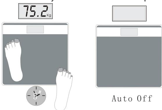
2. Stand steadily on the scale, it will switch on automatically and show the weight. The weight value will go to steady and be locked, when the unit appears following the weight value, and this is the result. For about 5 seconds after the unit appears, it will shut off automatically.
