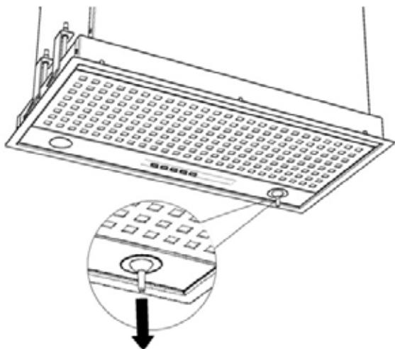
A suction cup for removing the lamps has been delivered with the hood. Place the suction cup onto the halogen spot and draw it towards you. The lamp will now come out. You can also install the new lamp using the suction cup.
