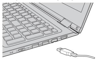
The first time you plug a USB device into a particular USB port on your computer, Windows automatically installs a driver for that device. After the driver has been installed, you can disconnect and reconnect the device without performing any additional steps.
