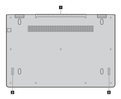
**Ventilation slots** Dissipate internal heat.
