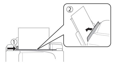
5. On the control panel, set the size and type of the paper you loaded in the rear paper feed.
