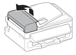
2. Use a soft, dry, clean cloth to clean the roller and the interior of the ADF.
