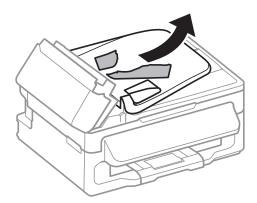
5. Raise the ADF input tray, and then remove the jammed paper.
