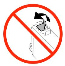
☐ Do not touch the sections shown in the illustration. Doing so may prevent normal operation and printing.
