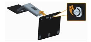
Attach the stand assembly to the monitor.
