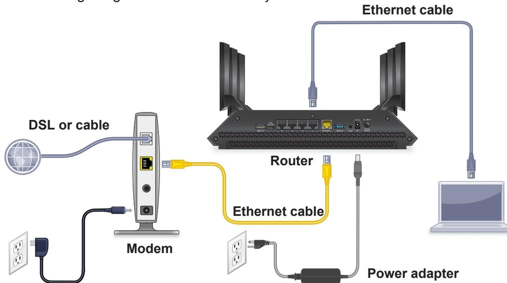
Figure 4. Router cabling
