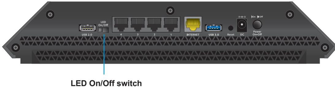
The Power LED stays lit even if the **LED On/Off** switch is in the Off position.
