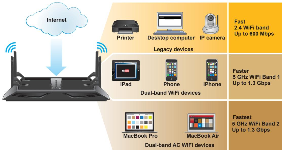
**Figure 9. Load balancing in a tri-band WiFi network**
