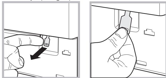
4. pull outwards using the tab as indicated in the figure, until the plastic tie-rod is freed from its stop position; pull downwards and open the door at the same time.
