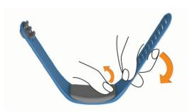
2 Insert the module into the replacement band.
