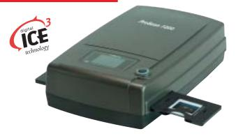
The ProScan 7200 provides an optical Resolution of 3600 dpi, a Dynamic Range of 3.8 Dmax and an extreme fast scanning time of 1 min 35 Sec for an colour scan with 3600 dpi and 48 Bit Colour Depth. The high scanning speed and also the hardware based dust and scratch removal system ICE contribute the ProScan 7200 to a very effective working tool. Using the attached slide and filmholder allows a high
