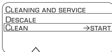
The **start** button **8** flashes while the different cleaning processes are running. The figures on the top right indicate the progress of the programme.
