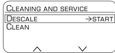
The **start** button **8** flashes while the different descaling processes are running. The figures on the top right indicate the progress of the programme.
