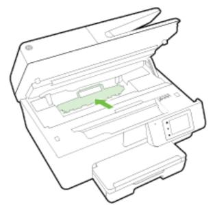
3. If the problem is not resolved, check the print carriage area inside the printer.
