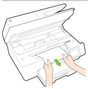
**b.** Move the carriage to the far left of the printer, and do the same as in the previous step to remove any torn pieces of paper.
