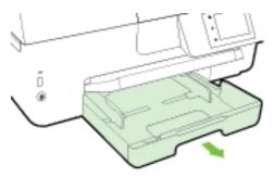
c. Press down the buttons on both sides of the input tray, and pull to remove the input tray.
