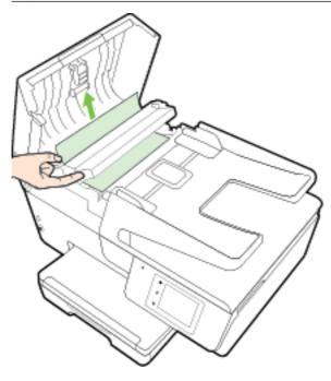
4. Close the document feeder cover, pressing down firmly until it snaps into place.
