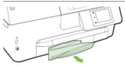
e. Insert the input tray, load paper, and lower the output tray.
