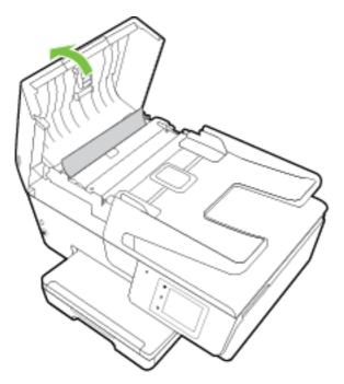
2. Lift the green tab located on the front edge of the document feeder.
