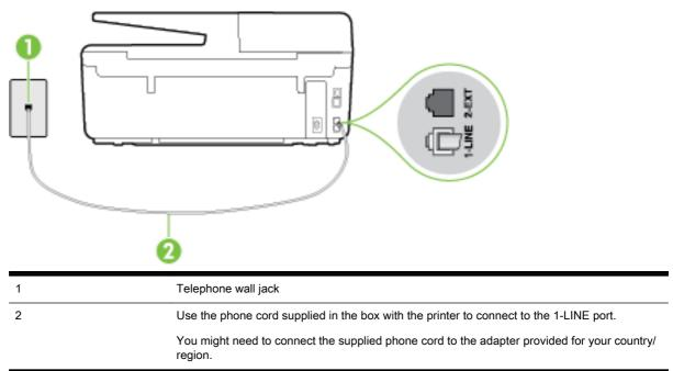
Figure B-5 Back view of the printer
