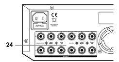
The connector terminals 24 "SPEAKER" for the six speakers are located on the back side of the receiver:
