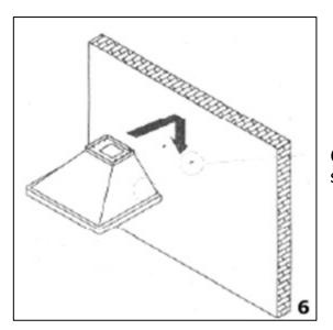
**6)** Hang the hood onto the support screws.
