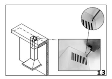
Slide chimney section (D) inside of chimney section (C). Then secure the L shaped bracket to the wall, using the same method as you have just used to secure the lower bracket.
