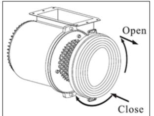
2) Press the carbon filter against one end of the motor, the fixing point is in the centre of the carbon filter.
