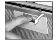
1) Remove the metal grease filters.
