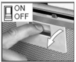
1) Remove the grease filters.
