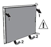
3. Hold the intermediate glass pane and unscrew the screw to remove the lower plate holding it in place.
