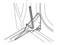
2. Grasp the door on both sides with both hands, lift it forming an angle of around 30° and remove it
