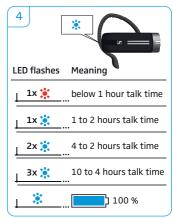
When the battery charge level drops below 15 minutes of talk time, the LED flashes red and the voice prompt "recharge headset" is announced several times. When the battery is flat, the headset switches off automatically.
