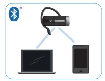
The headset complies with the **Bluetooth** 4.0 standard. In order that data can be transmitted wirelessly using **Bluetooth** technology, you have to pair your headset with **Bluetooth** devices that support the "hands free profile" (HFP), the "headset profile" (HSP) or the "advanced audio distribution profile" (A2DP).
