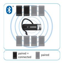
Only two out of the maximum eight paired Bluetooth devices can be simultaneously connected to the headset ("paired + connected").
