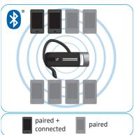
The headset can save the connection profiles of up to eight **Bluetooth** devices with which it has been paired. After switch-on, the headset automatically tries to connect to the two last connected **Bluetooth** devices. You can only connect a third **Bluetooth** device after having switched off the first or the second **Bluetooth** device.
