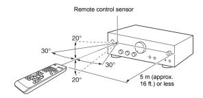
When using the remote control, point it toward the remote control sensor on the unit from a distance of 5 m (approx. 16 ft.) or less.
