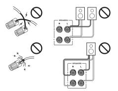
(North American models) When using commercially available banana plugs, tighten the speaker terminals to the end and then insert the banana plugs. It is not possible to connect by inserting the core of the speaker cable directly into the hole for a banana plug. Make sure to attach a banana plug before inserting.
