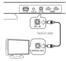
2. Set the INPUT source to OPTICAL. Press repeatedly **FUNCTION** on the remote control or **F** on the unit until the function is selected. For selecting directely the OPTICAL function, press **OPTICAL** on the remote control.
