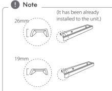
Install proper cover foot of either 19mm or 26mm in height to match the unit to the underpart of TV screen at the suitable level. (26mm cover foot has been already installed to the unit.)
