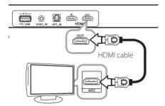
2. Turn TV and the unit on. ARC function is selected automatically.
