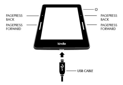
**PagePress**: To page forward or back in a book, squeeze either side of the screen. Use the line to page forward, and the dot to page back. You can keep your right or left thumb resting on the pressure-sensitive controls. To adjust the pressure required to turn a page, or
