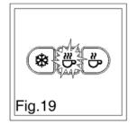
Fig.19 When the  $\overset{{w}}{\bigcirc}$  light is flashing this indicates a problem with the thermostat of the appliance. Please switch off the electricity supply and inform the service department.
