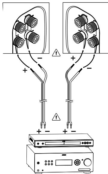
**⑥ Setup B - bi-wiring
