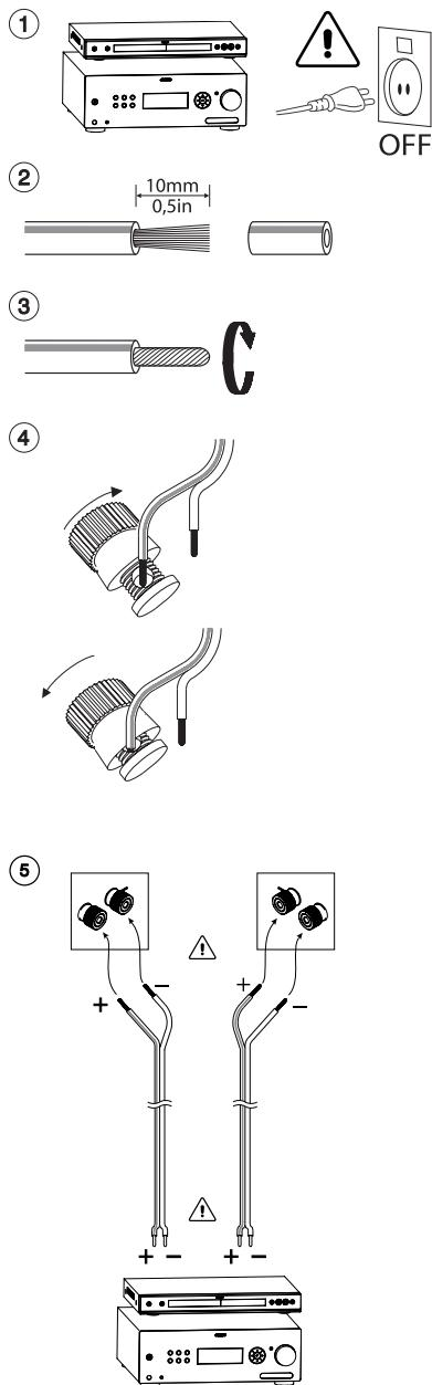
**⑥ Setup A - single wiring
