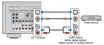
If you select the input source by pressing AV 1–6, the audio played back on the audio device will be output from the unit.
