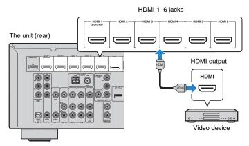
If you select the input source by pressing HDMI 1–6, the video/audio played back on the video device will be output from the unit.
