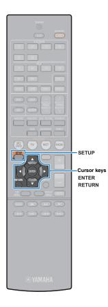
To start the measurement, use the cursor keys to select "Start" and press SETUP.
