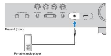
If you select "AUX" as the input source by pressing AUX, the audio played back on the device will be output from the unit.
