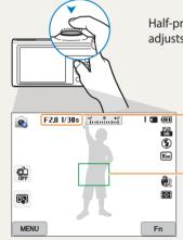
Half-press [**Shutter**] and adjust the focus. The camera adjusts the focus and exposure automatically.
