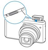
While not in use, keep the flash unit closed to prevent damage.
