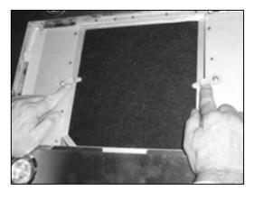
3) After inserting the front edge of the carbon filter into the slot on the cooker hood. Lower the back edge of the carbon filter, until it clicks into place at the rear of the rectangular hole. Raise the two fixing bars, until they are horizontal over the carbon filter.
