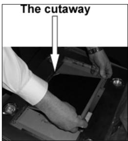
2) Insert the carbon filter in the rectangular hole, fitting it over the motor.
